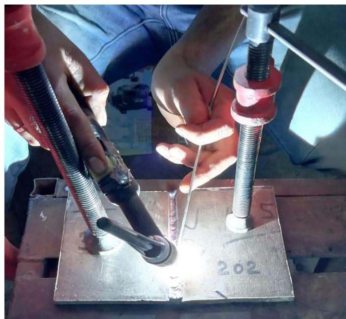
Figure 1: Tungsten inert gas welding during process
